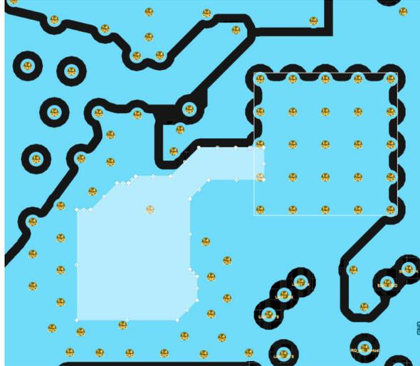
**Figure 3-12. Reference Layout for Layer Under XTAL Cutout**
