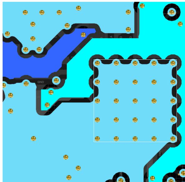
Figure 3-14. Reference Layout of the Power Layer
